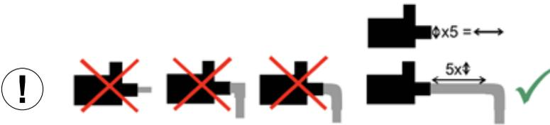
If the intake line is longer than 10 meters or the intake height is higher than 1 meter, the diameter of the intake line must be bigger than the inlet of the pump.
